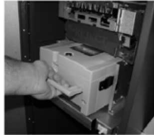
Removing note tray from the dispensing mechanism.
